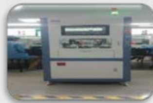
Name: AUTOMATIC SCREW MACHINE Function: It tightens the screws on mobile with specific torque values
