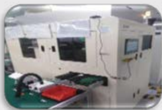
Name: DECO BRACKET PASTING. Function : It place the deco on the mid shell.
