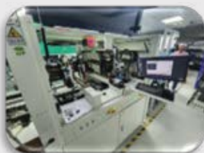
Name: AUTOMATIC GLUE DISPENSING Function: It applies the glue to the shell & check the quality with 3D scanning
